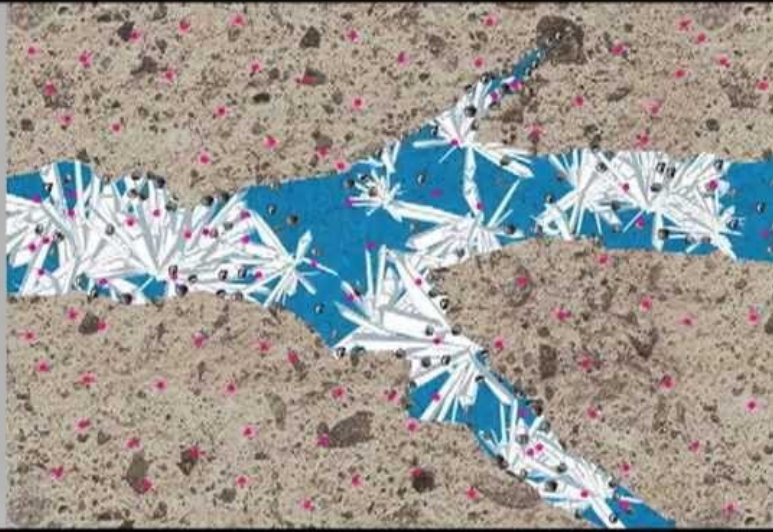
11 The Xypex Crystalline Technology can also be applied as an admixture to the concrete at the time of batching. In this case the Xypex active ingredients are evenly dispersed throughout the cement matrix with slightly higher concentrations in the capillary water.
