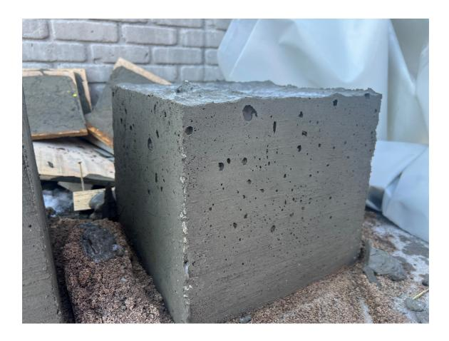
The final cube exhibited a significant amount of bugholes and honeycombing. Additionally, a great deal of paste was lost through the corners of our admittedly-not-expertly-built forms, resulting in a lower mass of concrete still in the forms and edges of the cube that were not uniform. By over-vibrating, we actually
