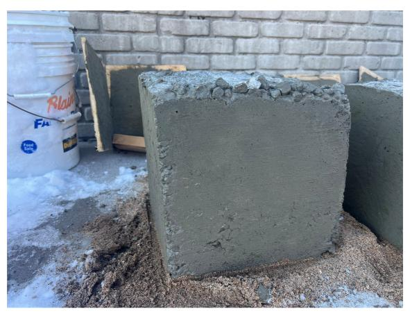
As you can see, the first cube does not have a clean corner and the higher elevation of the concrete suggests air voids present throughout the concrete. There is also quite a bit of rough surface near the bottom of the cube.
