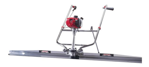
Surface vibrating screeds such a laser screed, truss screed, or vibra-screed utilize vibration to consolidate the concrete as it is screeded and bring up cream to aid in workability.
