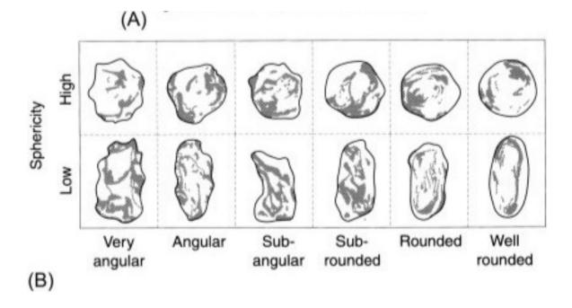
Aggregates, particularly fine aggregates, that are angular or elongated are very difficult to pump. Rounded fine aggregates like natural river sands are a huge advantage in creating a pumpable concrete mix.
